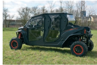
POLYCARBONATE CABIN FULLY ACCESSORIZED (wiper/washer asm./heater asm.) M64S07U04-0
